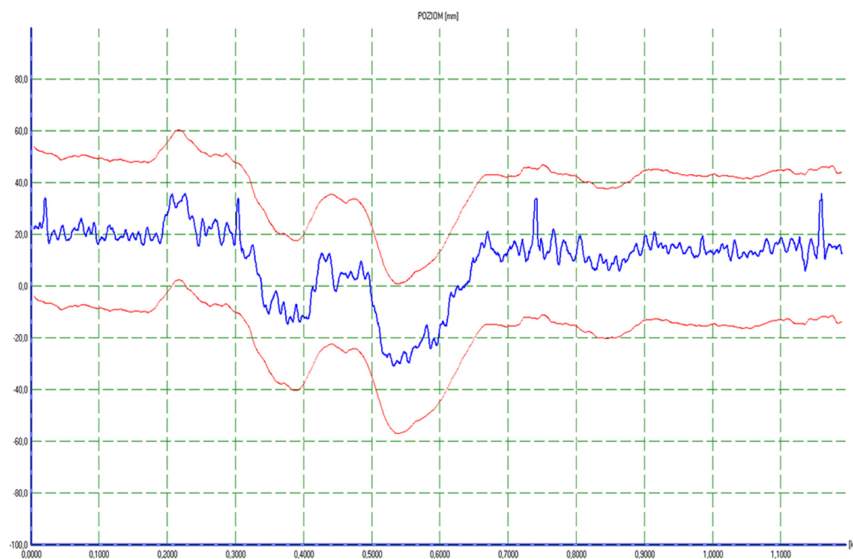
Fig. 2. An example of the chart of horizontal sagittas obtained with an electronic track gauge (on the horizontal axis – distance (m), on the vertical axis – sagitta values (mm), the red lines indicate the tolerance limits for the speed 50 km/h)
