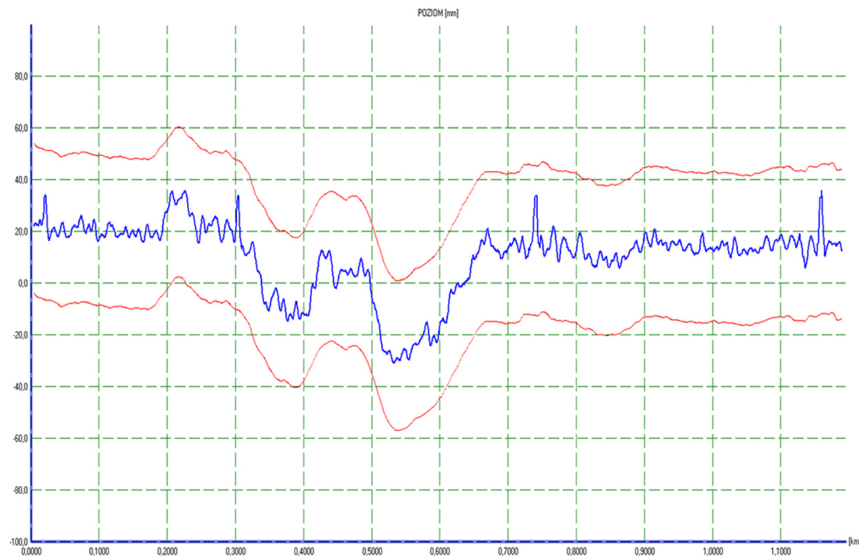
Fig. 2. An example of the chart of horizontal sagittas obtained with an electronic track gauge (on the horizontal axis – distance (m), on the vertical axis – sagitta values (mm), the red lines indicate the tolerance limits for the speed 50 km/h)
