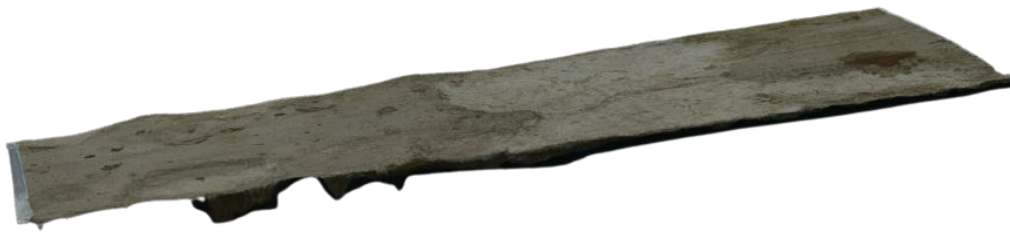
Figure 9. An example of a scan of the corroded surface (specimen 6.3).
