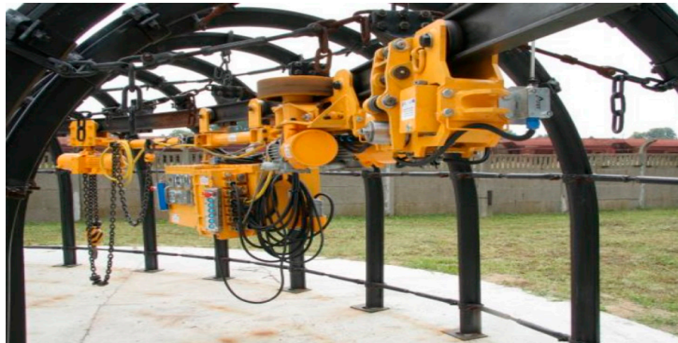
Figure 3. Operation of a suspended battery vehicle (PCA-1).
