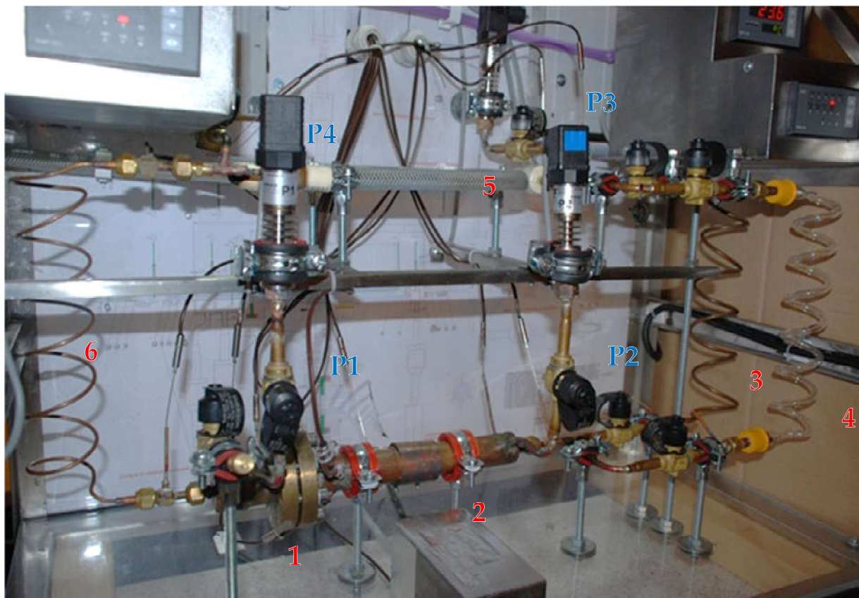
Figure 9. Photograph of the test facility with marked measurement points (before insulation): 1—compensation chamber; 2—evaporator; 3—vapour line; 4—glass tube for inspection of flow structure in vapour line; 5—condenser; 6—liquid line; P1, P2, P3, P4—pressure transducers.
