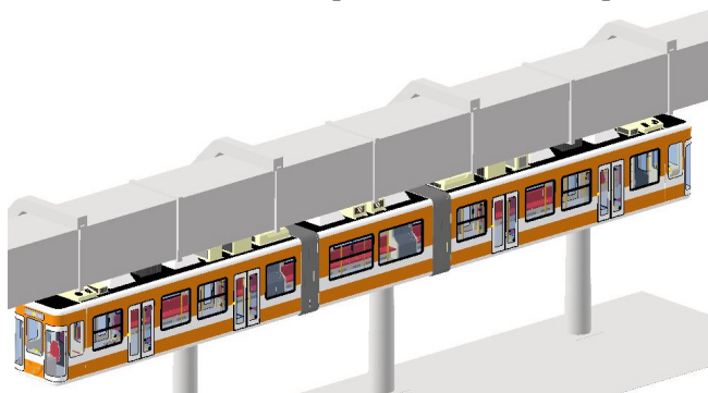
Fig. 1. Authors' suspended electric multiple unit [5]
