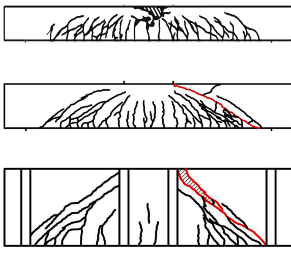
Fig. 5. Crack patterns at failure typical for RC beams with stirrups (series '4') [22]: a) beam S4D22A108 ( \eta_a = 5.0 ), b) S4D43A108 ( \eta_a = 2.5 ), and c) S4D72A108 ( \eta_a = 1.5 ).
