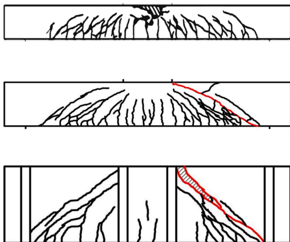
Fig. 5. Crack patterns at failure typical for RC beams with stirrups (series ‘4’) [22]: a) beam S4D22A108 ( \eta_a = 5.0 ), b) S4D43A108 ( \eta_a = 2.5 ), and c) S4D72A108 ( \eta_a = 1.5 ).
