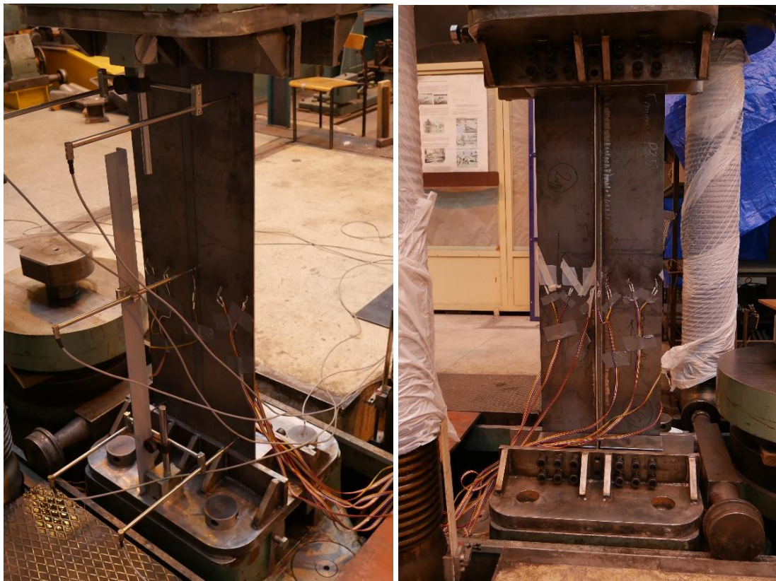
Figure 6.15. Back (left) and front (right) view on the specimen with installed gauges.
