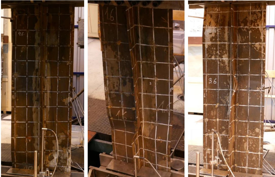
Figure 6.48. Post-collapse shapes for 6 mm specimens with degradation level of 7% (left), 14% (mid) and 21% (right).
