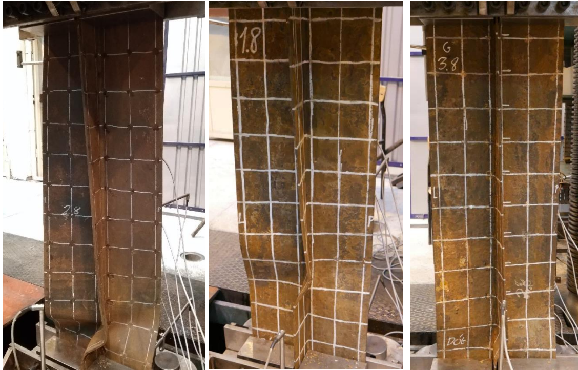
Figure 6.49. Post-collapse shapes for 8 mm specimens with degradation level of 7% (left), 14% (mid) and 21% (right).
