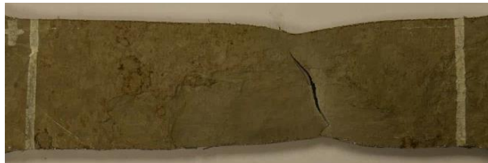
6.10 specimen – FE (top) and experimental (bottom) failure mode
