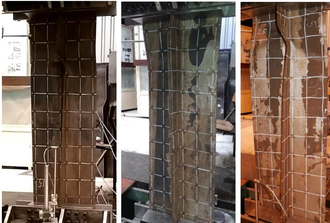
Figure 6.46. Post-collapse shapes for 5 mm specimens with degradation level of 7% (left), 14% (mid) and 21% (right).
