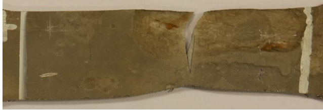
5.4 specimen – FE (top) and experimental (bottom) failure mode
