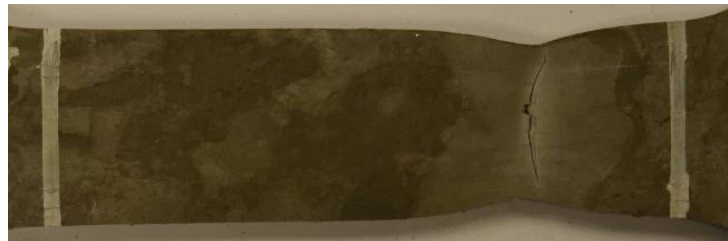
8.10 specimen – FE (top) and experimental (bottom) failure mode
