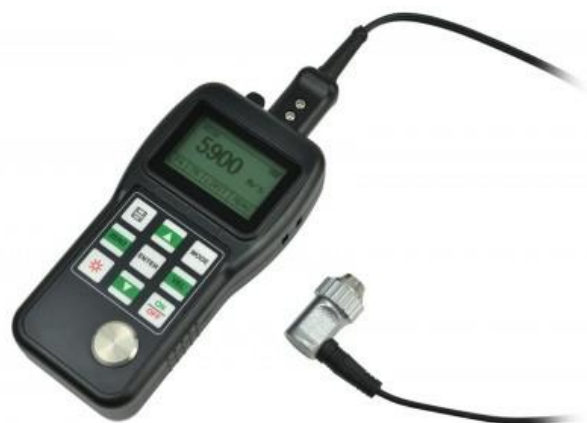
Figure 4.6. Typical ultrasonic thickness gauge.
