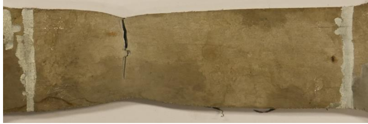
8.8 specimen – FE (top) and experimental (bottom) failure mode
