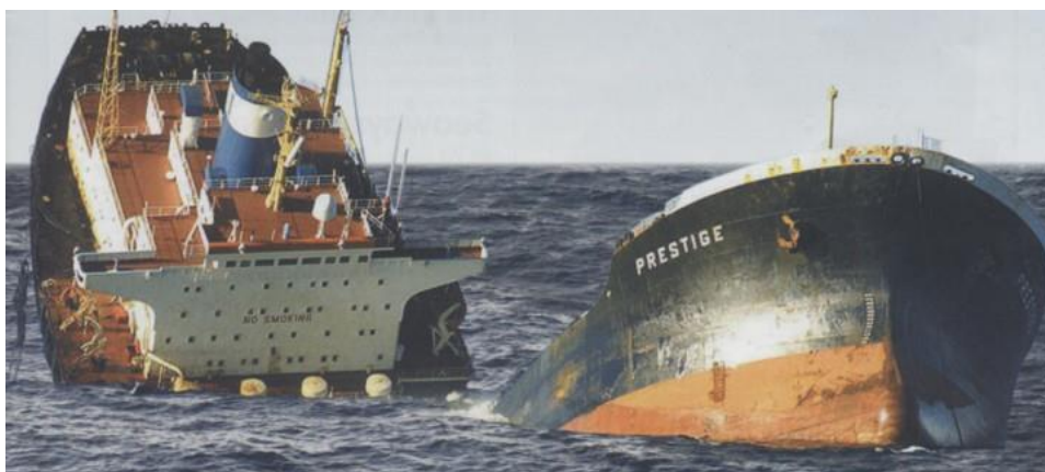
Figure 1.4. Breaking of tanker ship Prestige [10].
