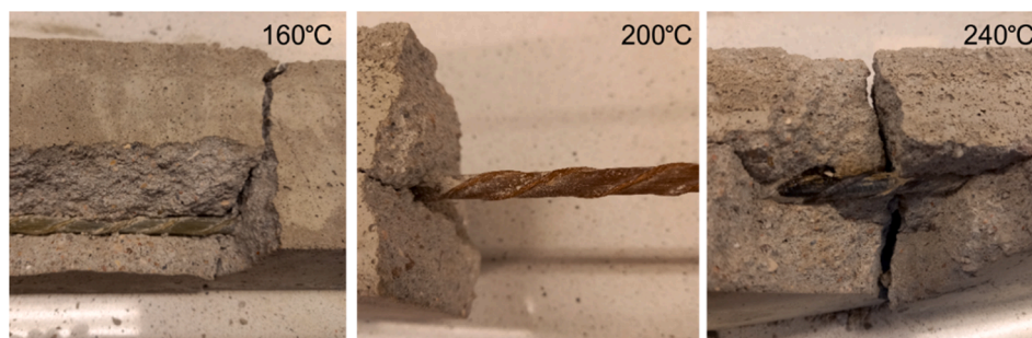
Fig. 8. Uncovered GFRP reinforcement after destructive bending tests.
