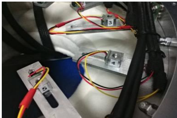
Fig. 5. Cantilever beams (5 out of 8) inside REXUS 25 rocket [11].
