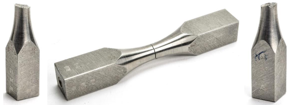
Figure 1. The real S355J2 steel specimen after fatigue test.
