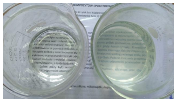
Fig. 2. Comparison optical transparency, a) neat diesel fuel b) nanofuel – \text{Al}_2\text{O}_3 50 ppm, turbidity ~30 NTU
