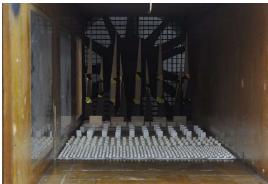
Figure 3. View from inside the tunnel with elements used to model the boundary layer.
