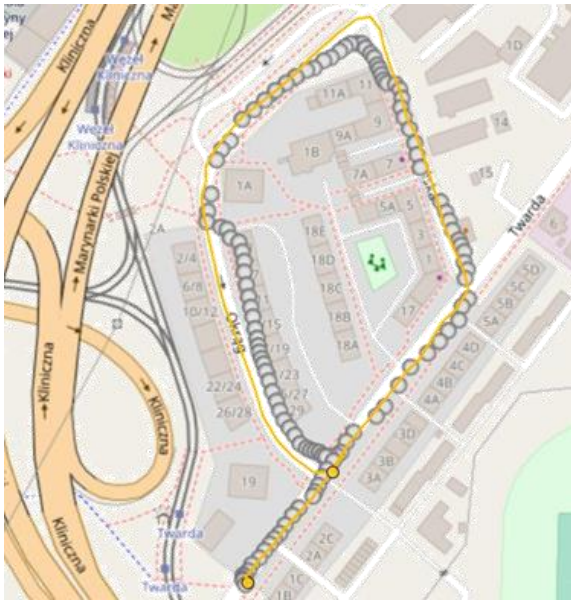
Fig. 7. Car excursion along the square-shaped route with smartphone 2: yellow – real route, dot – measured route
