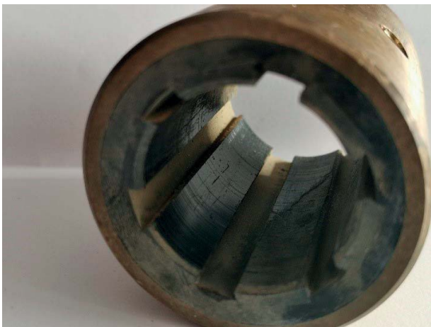
Fig. 5. The PTFE sliding bush (B)
