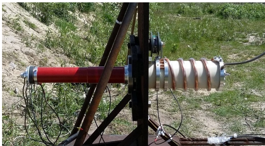
Figure 15. Photograph of the integrated high-power pulse generation and forming system field test stand with the armor plate protecting the FF and measuring transducers against FCG explosion.
