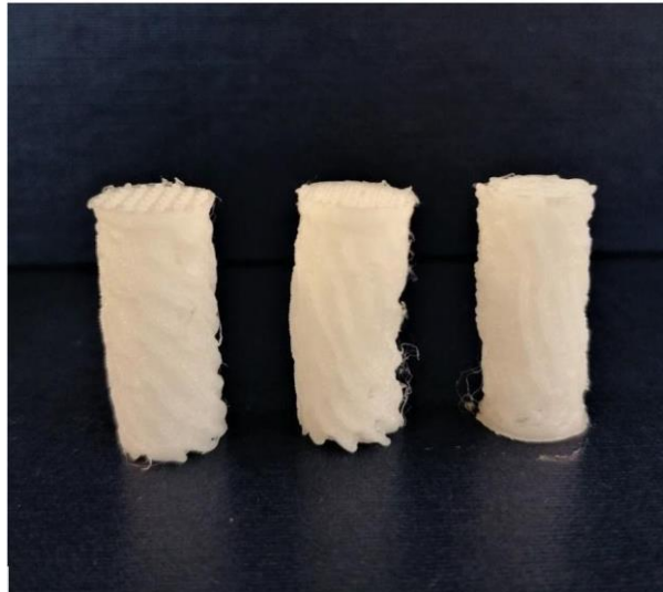
Fig.6. The photography of 3D objects in the form of cylinders printed with the FDM method from the obtained composite filaments (from the left 3D prints containing 5%, 10% and 15% of chitosan).
