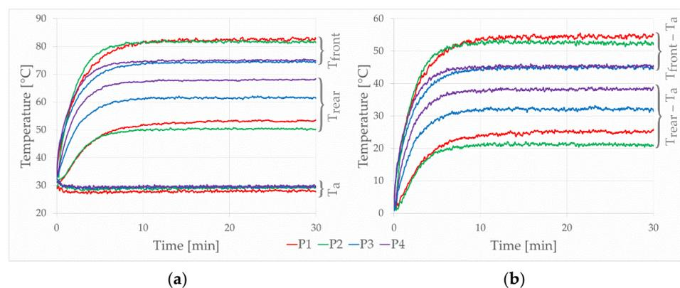
**Figure 5.** Module (a) front, rear, and ambient temperatures (b) front and rear temperature related to ambient temperature during tests.**Table 6.** Front and rear temperature related to ambient temperature at the end of the measurement and time constant for each prototype.
