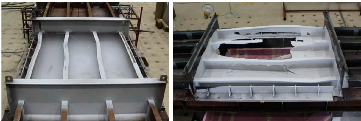
Figure 8. The stiffened panel collapsed at -80^{\circ}\text{C} (Paik et al., 2021a) (left) and at cryogenic conditions (Paik et al., 2020a) (right).
