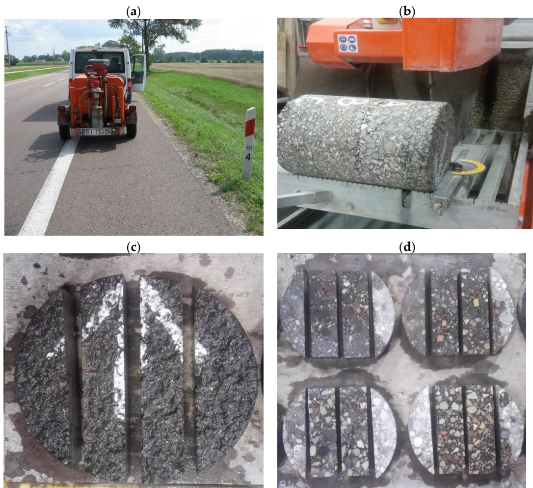
Figure 4. The method of specimen preparation: (a) core specimens drilled from road sections, (b) division of cores into individual layers, (c) cutting along the direction of vehicle movement, and (d) formation of prismatic beams.
