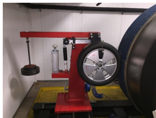
Figure 3. Roadwheel facility for tire rolling resistance measurements.
