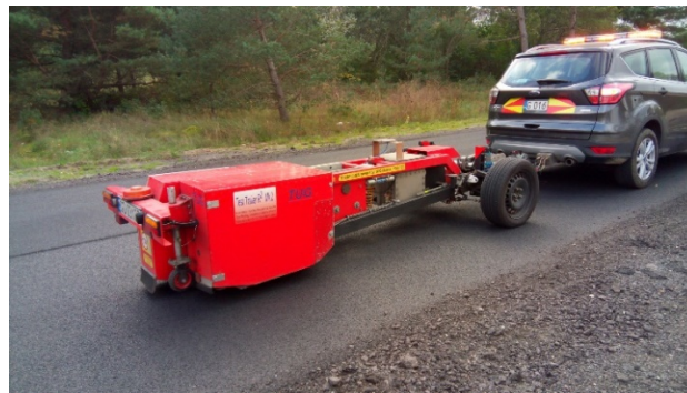
Figure 4. Test trailer R 2 Mk.2 for tire rolling resistance measurements.
