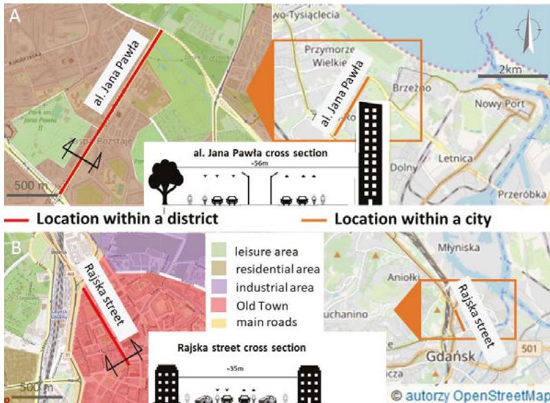
Fig. 1. Location of Gdansk's cycle lanes ( www.gdansk.pl , google.com ) and street cross-section of analysed roads ( streetmix.com )
