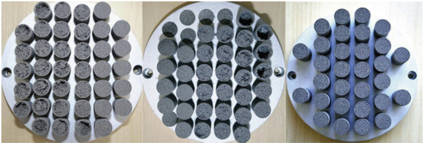
Figure 4. Porous samples made for permeability measurements [25].
