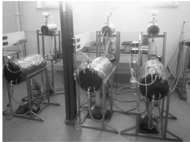
Figure 2. Reactors for carrying out research on the methane fermentation process.
