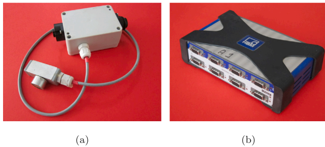
Fig. 21. (a) Tri-axial micro-electro-mechanical capacitive accelerometers (MEMS) accelerometer; (b) QUANTUM HBM 840a eight-channel measurement amplifier.
