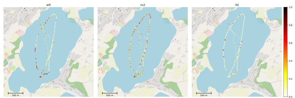
Figure 12. MAVLink message loss ratio measurements for Wi-Fi, NV2 and RFD devices.
