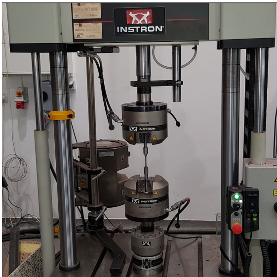
Fig. 2 Servo-hydraulic machine used to carry out the fatigue tests
