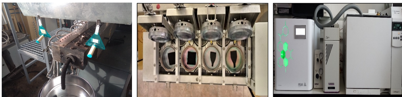
Figure 5. The appearance of the apparatus for determining the TVOCs parameter; from left: Radiello® passive sampling system; Micro-Chamber/Thermal Extractor™; gas chromatograph.
