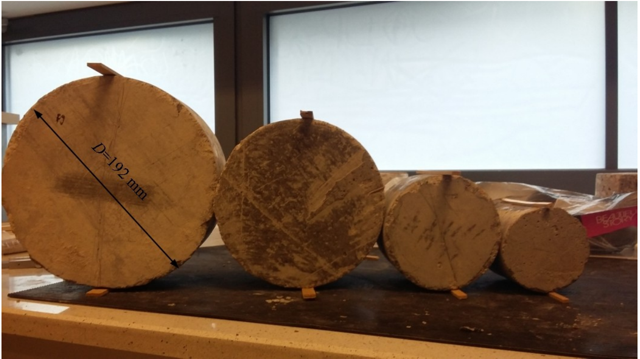
Fig.3.25: The specimens with plywood strips scaled proportionally with specimens diameter ( b/D=\text{const.} )
