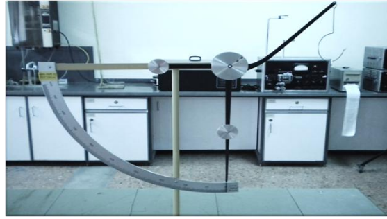
Fig. 142: The view of square meter balance device, used for measuring in the laboratory photo by author
