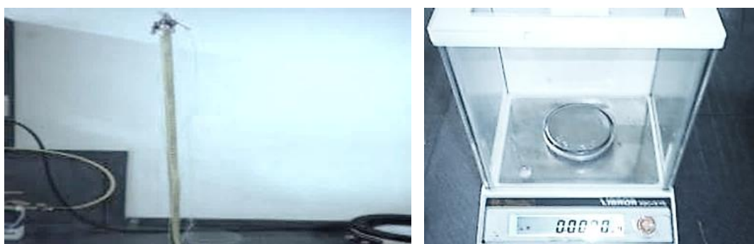
Fig. 145: Place of hanging yarn from the hook, digital scale with 4 decimal places for weighing yarns, laboratory photo by author
