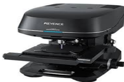
Rys. 5.29. Mikroskop laserowy (Keyence 3D Laser Scanning Confocal Microscope VK-X Series) [108]
