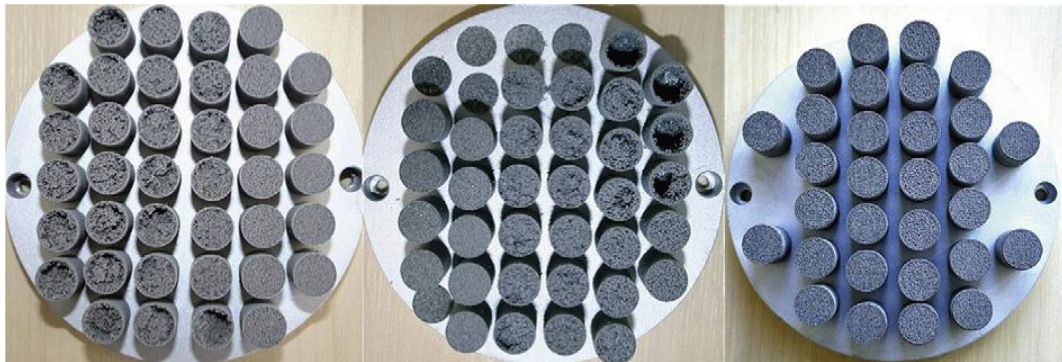
Figure 2. Additively manufactured porous wick samples [12].
