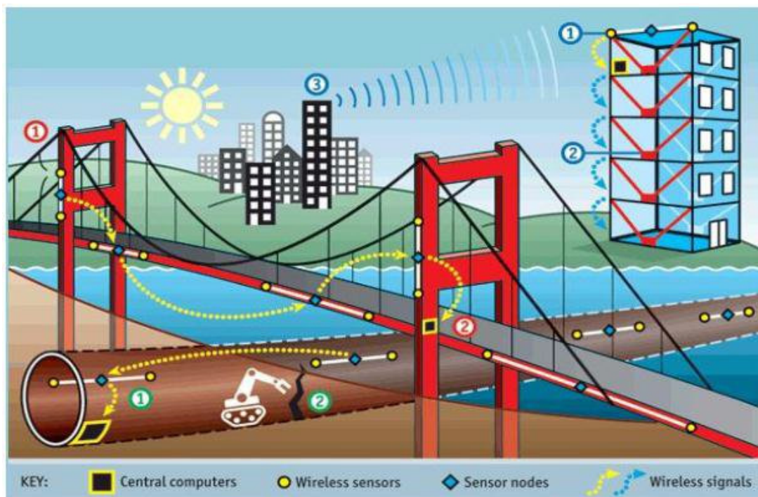
Figure 7. Civil engineering structures equipped with SHM systems using wireless sensor networks [52].
