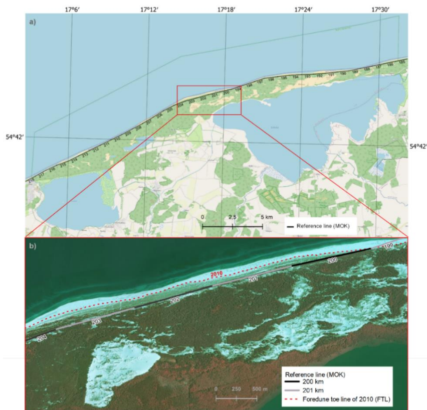
Figure 3. The route of the reference line (RL)—Polish Maritime Office’s Kilometer line (MOK), (a) along the examined coast section of the Baltic Sea, the base map—OpenStreetMap, (b) The routes of the selected part of RL and FTL line in year 2010 (red color)—the base map—orthophotomap dated 2010.
