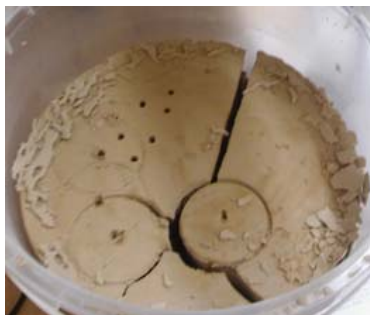
Fig.2. Effects of bentonite drying-out inside the bucket. Cracks and shrinkage of the bentonite from the bucket wall toward the center progressed within approx. 2 weeks of making the sample
