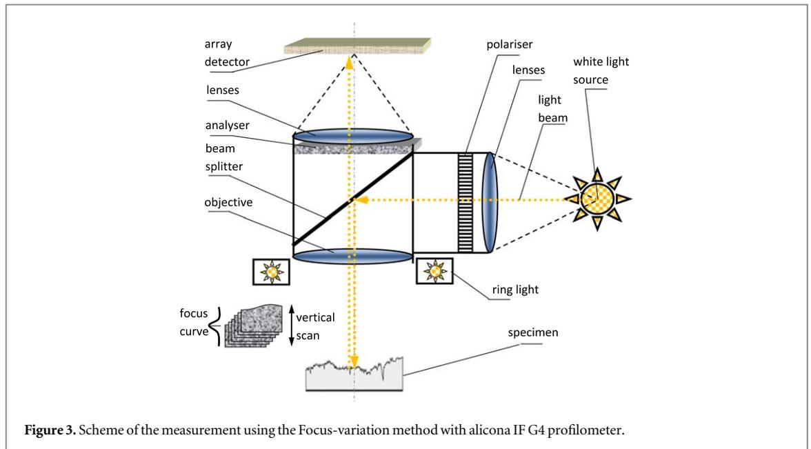
Figure 3. Scheme of the measurement using the Focus-variation method with Alicona IF G4 profilometer.
