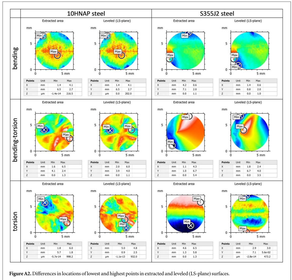
Figure A2. Differences in locations of lowest and highest points in extracted and leveled (LS-plane) surfaces.
