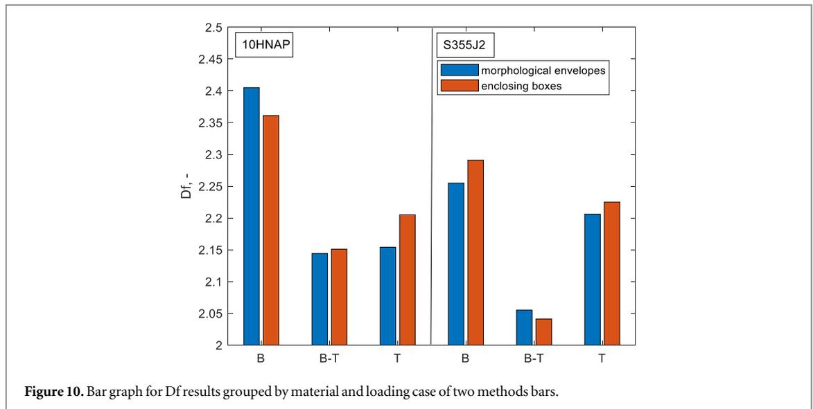
Figure 10. Bar graph for Df results grouped by material and loading case of two methods bars.
