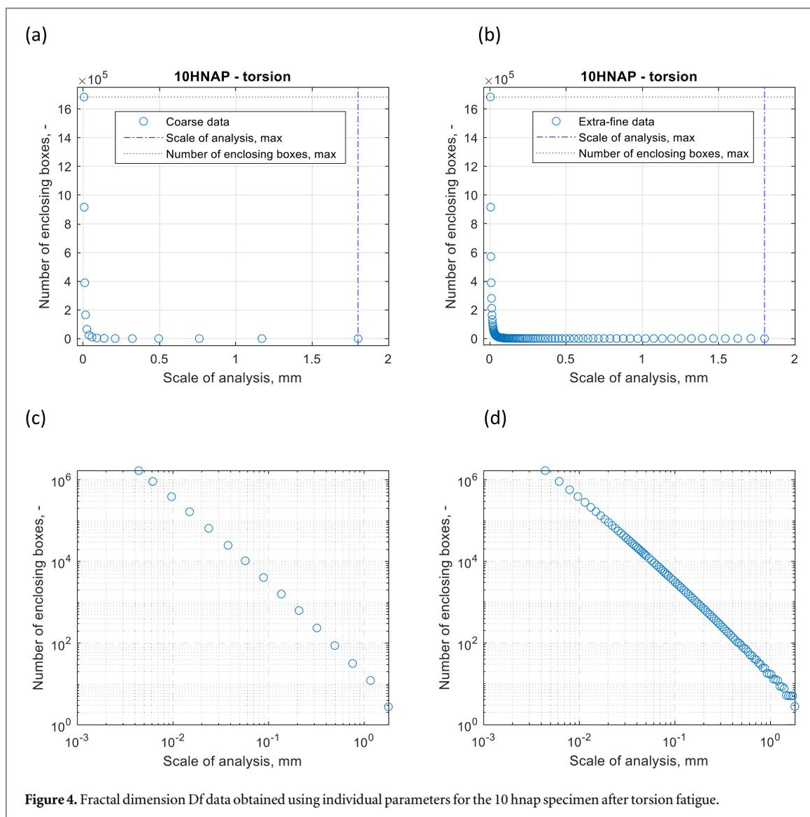
Figure 4. Fractal dimension  $D_f$  data obtained using individual parameters for the 10 hnap specimen after torsion fatigue.
