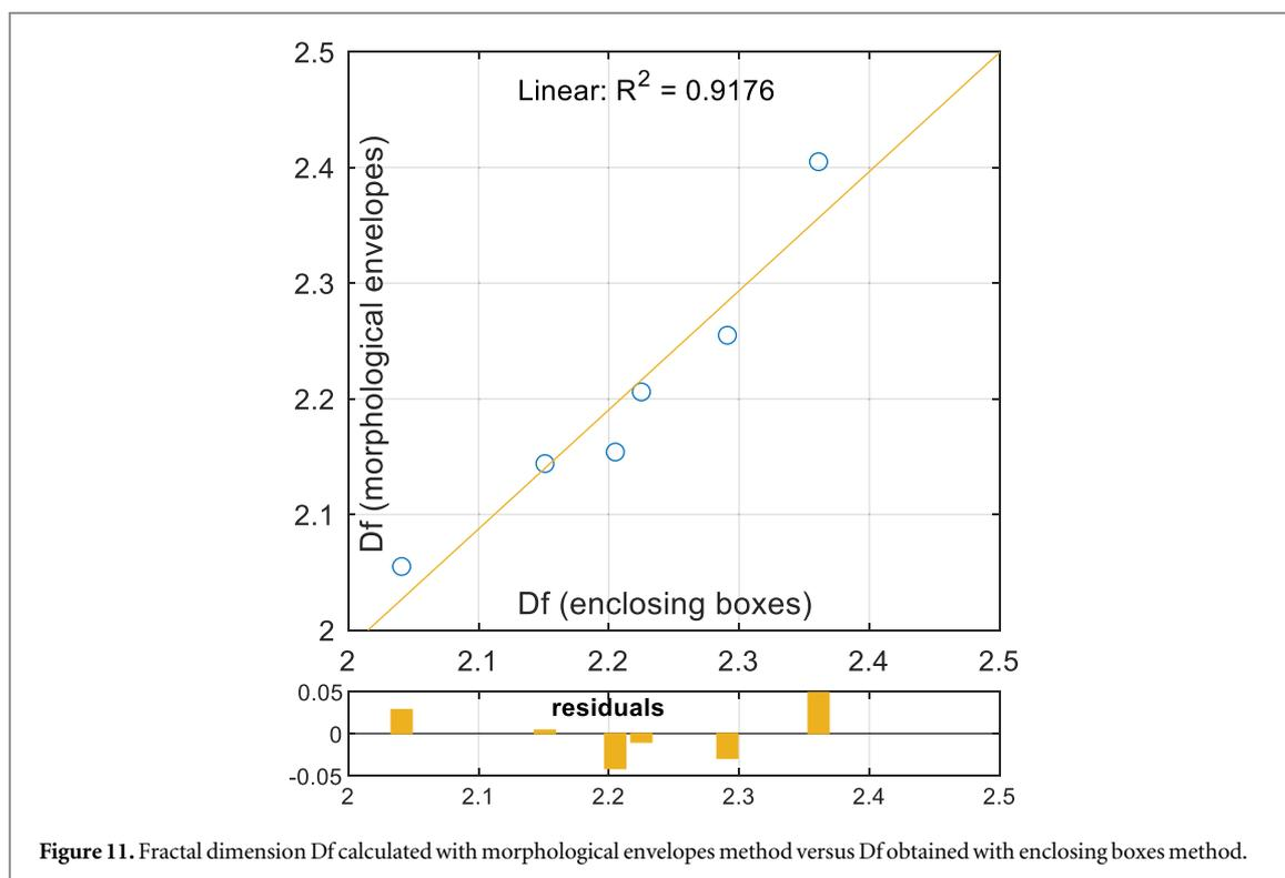
Figure 11. Fractal dimension  $D_f$  calculated with morphological envelopes method versus  $D_f$  obtained with enclosing boxes method.
