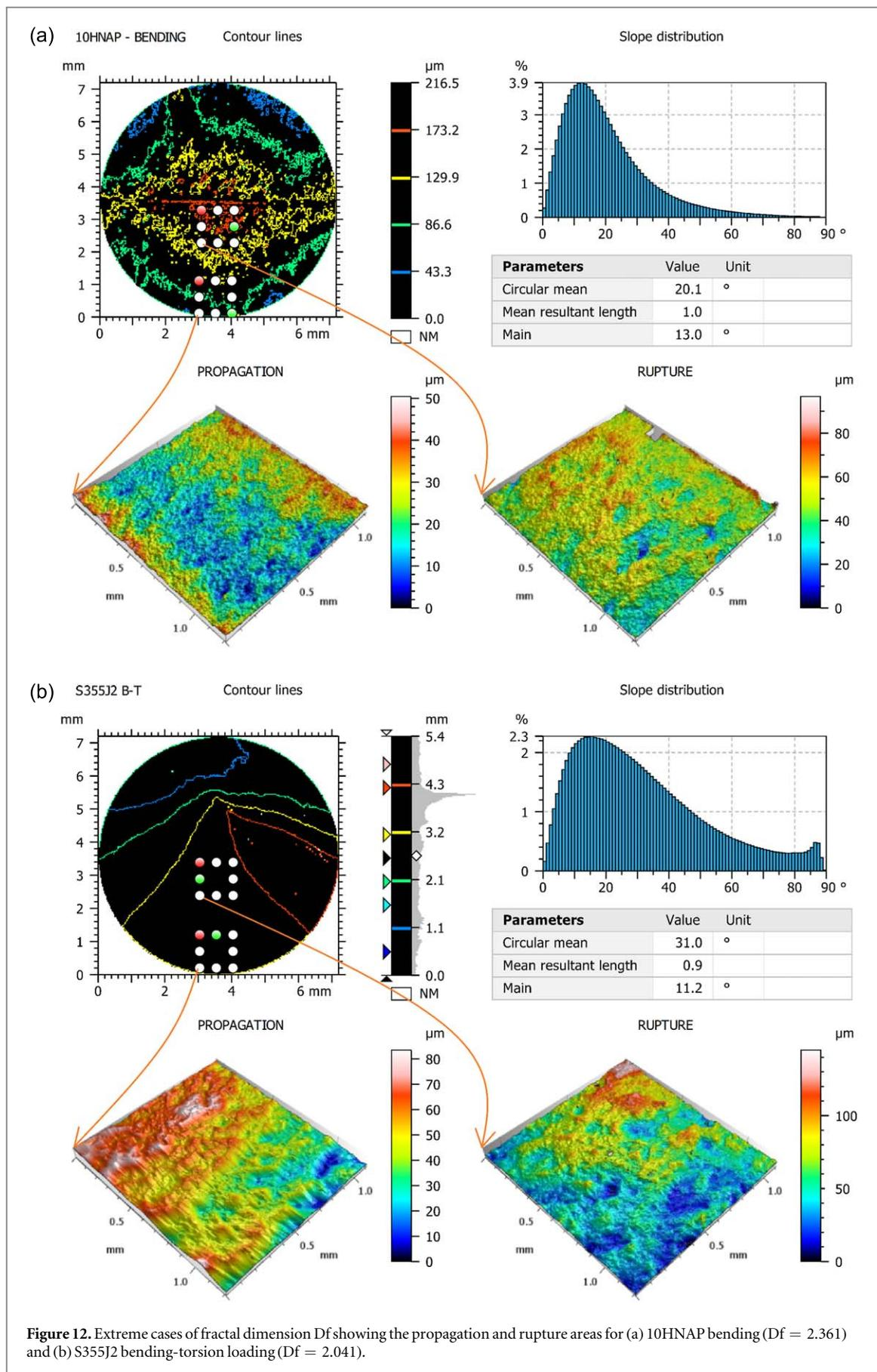
Figure 12. Extreme cases of fractal dimension  $D_f$  showing the propagation and rupture areas for (a) 10HNAP bending ( $D_f = 2.361$ ) and (b) S355J2 bending-torsion loading ( $D_f = 2.041$ ).
