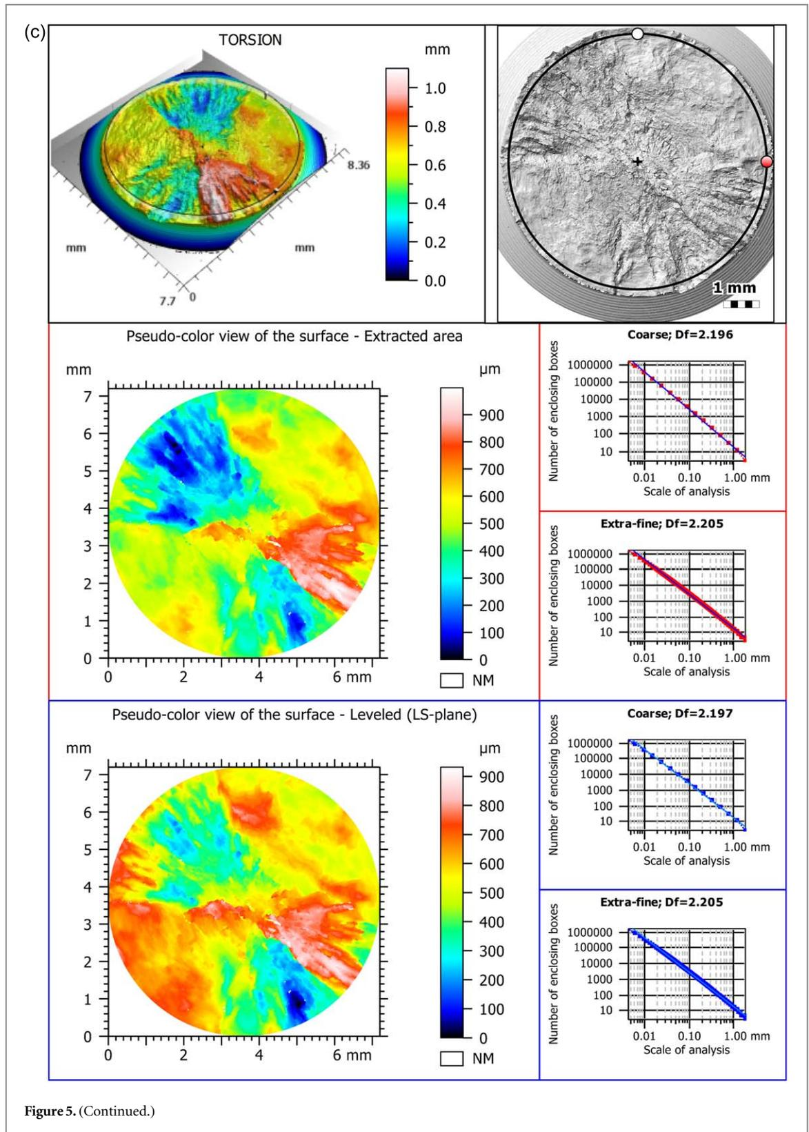
Slope and coefficient of determination  $R^2$  are calculated for two regression lines, one connecting the points to the left of the graph, the other connecting the points to the right (see figure 7). This makes it possible to analyze multi-fractal curves with two different slopes depending on the scales in the analysis. The fractal dimension Df is determined with a greater  $R^2$  value. Figure 7 shows
