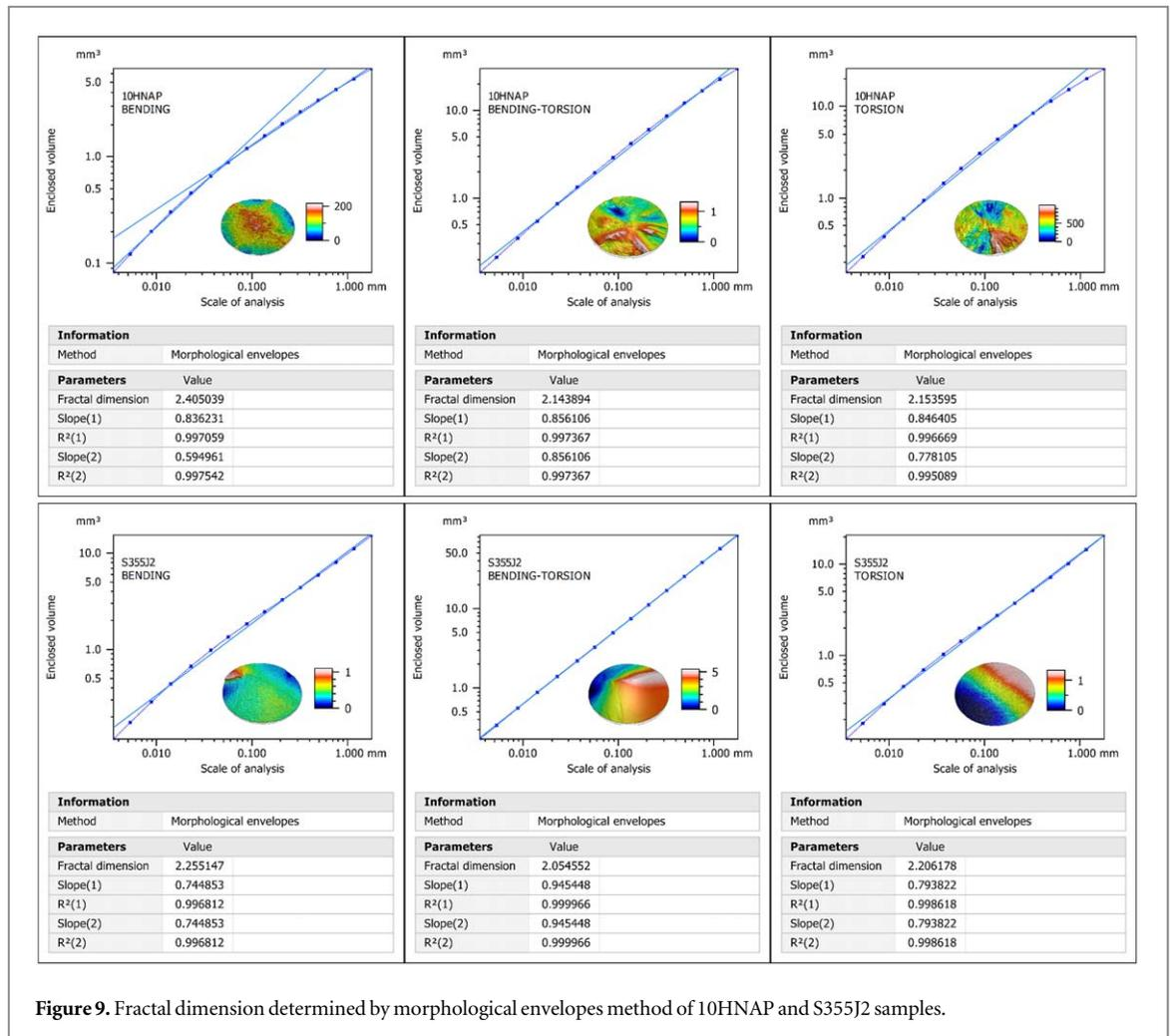
Figure 9. Fractal dimension determined by morphological envelopes method of 10HNAP and S355J2 samples.
