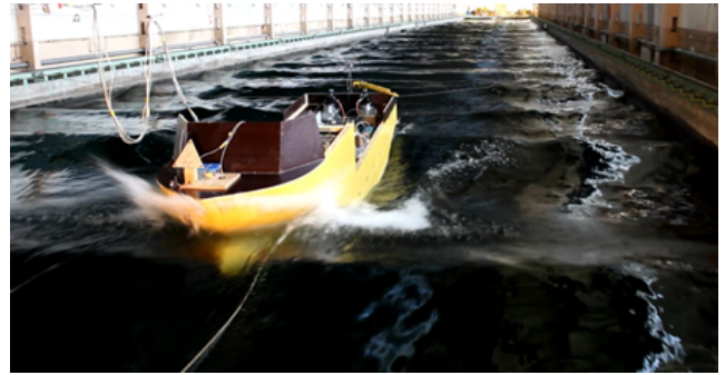
FIGURE 1. The reduced-scale free-running model of ship in the deepwater towing tank at the Maritime Advanced Research Centre [40].
