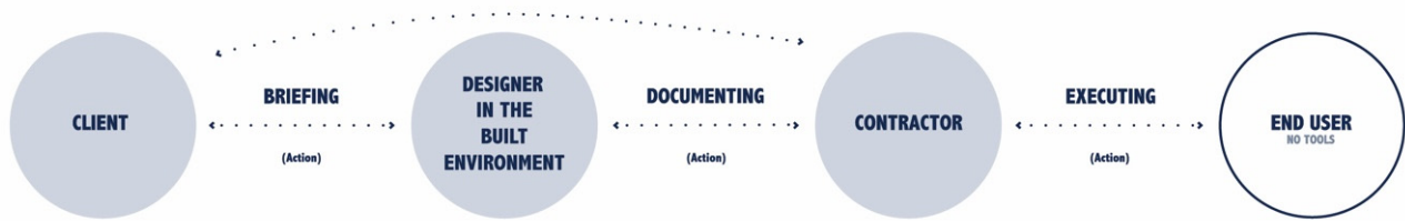
Figure 10. The current linear design process of an urban lighting project. Source: authors' own work based on experts' opinions.
