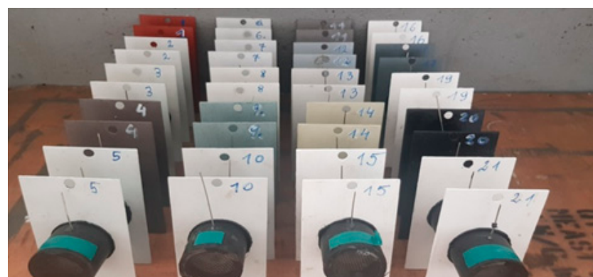
Figure 3. Additional detachable coating samples before assembly on the ball mill and in the hall with glued-on measuring cells for impedance measurements.
