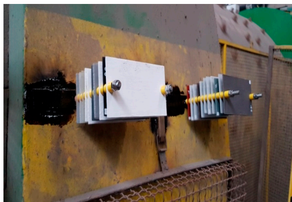
Figure 4. Mounted coating samples on the body of the ball mill (presence of vibration).
