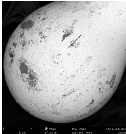
Figure 1. SEM image of the microsphere-sensor with a 100-nm ZnO Atomic Layer Deposition (ALD) coating. Magnification of 1000 \times .
