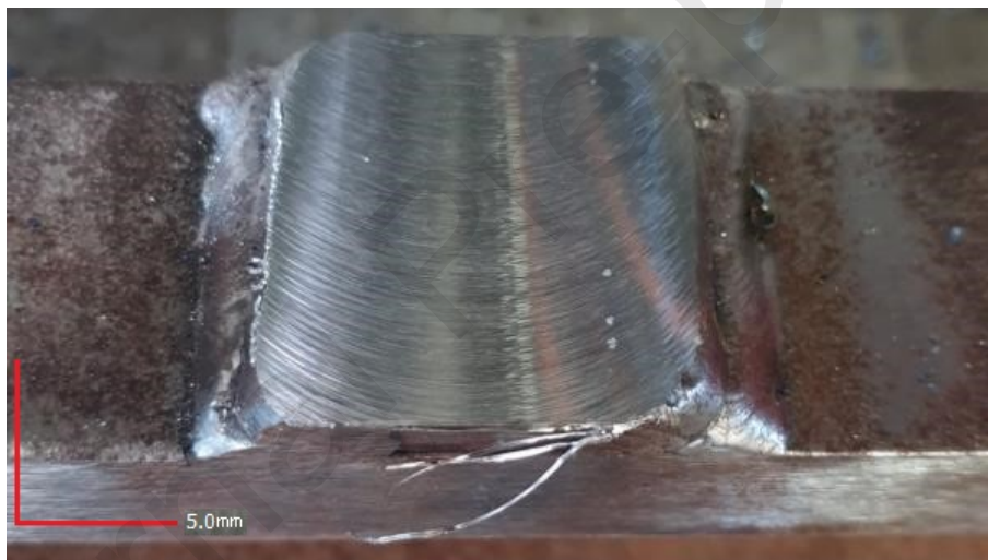
Figure 9. Cavity observed in triple weld specimen.
