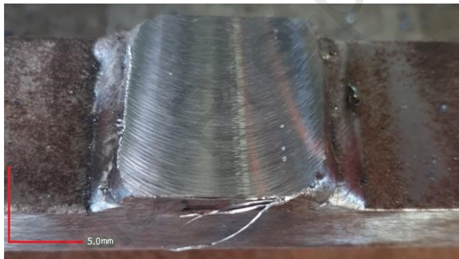
Figure 9. Cavity observed in triple weld specimen.
