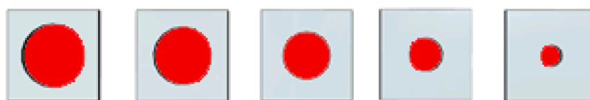
Scheme 1. Masks applied to CB-PLA electrodes to partially cover the surface area prior to activation.
