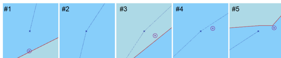
Figure 8. Graphic rendering of the determination of the decision function value (magenta—GNSS, dark blue—calculated position, blue—safe area for navigation, light blue—dangerous area for navigation).
