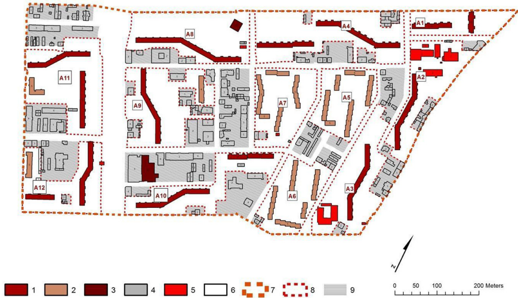
Figure 1. Typology of built structures of the Zgierska-Stefana estate, Bałuty, Lodz. Notes: (1) Twelve-floor wave blocks; (2) four- or-five-floor blocks of flats; (3) tower buildings; (4) auxiliary structures; (5) services, (6) buildings in the historical parts; (7) site limits; (8) historical development; A1–A12 are unit IDs.
