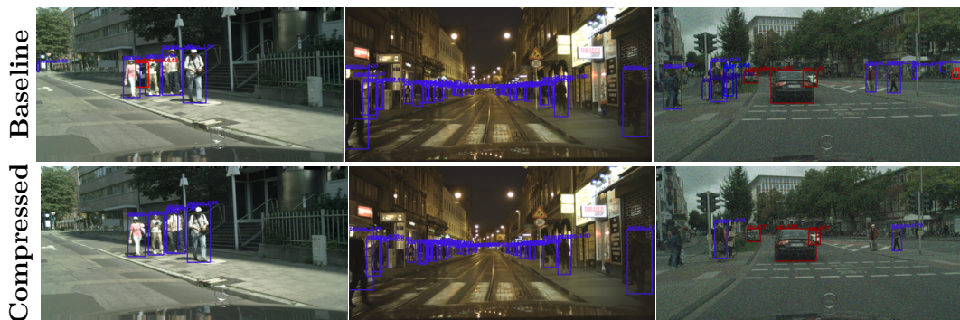
Figure 4.5: Detection samples for the baseline model and the model structurally pruned at 70% compression rate. Detections on the original Cityscapes dataset (first column), ECP dataset (second column) and noise distortion (third column).
