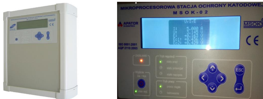
Figure 4. View of the MSOK-02 microprocessor cathodic protection station and its control panel.
