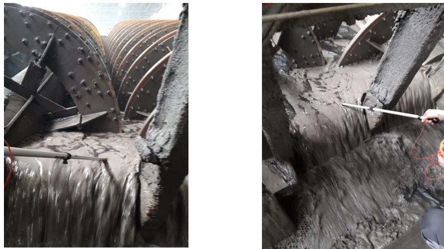
Figure 12. Verification measurements of the classifier spiral potential using a portable electrode.
