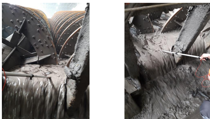
Figure 12. Verification measurements of the classifier spiral potential using a portable electrode.
