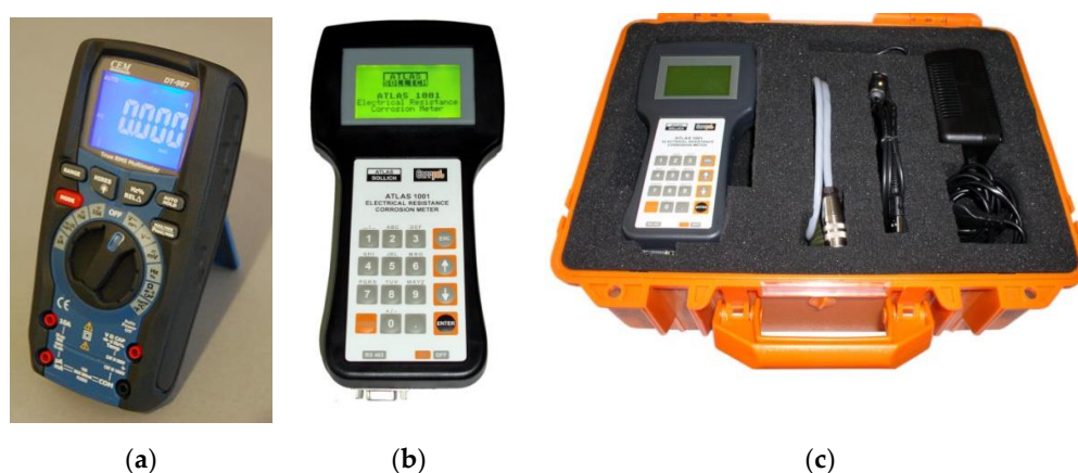
Figure 11. Meters fitted in the protection system: (a) multimeter for potential measurements, (b,c) ATLAS 1001 COR resistive corrosion meter with accessories.
