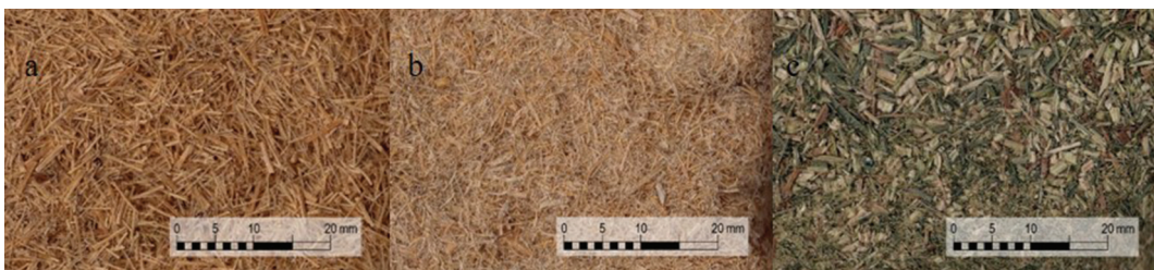
Figure 1. Pictures of materials obtained (from left to right): (a) fibers from stems, (b) fibers from leaves, and (c) shredded material.
