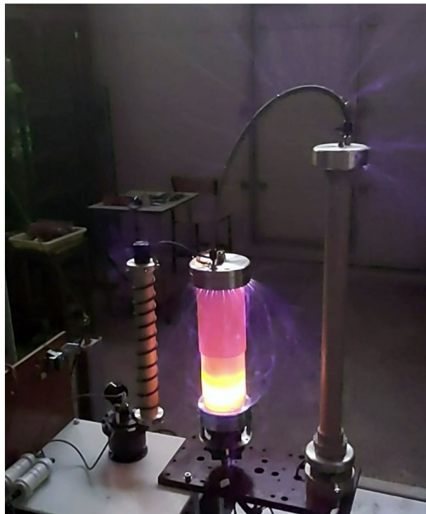
Figure 18. View of partial discharges of volatile nature in the space around the TSFF model, voltage divider, and the upper fitting of the forming coil during the pulse forming process (for the overvoltage peak value U_{max} = 740 kV).
