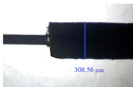
Figure 1. Image of the produced SPME fiber (on the left side, a glass core can be seen) magnified by 50×, and respective diameter.
