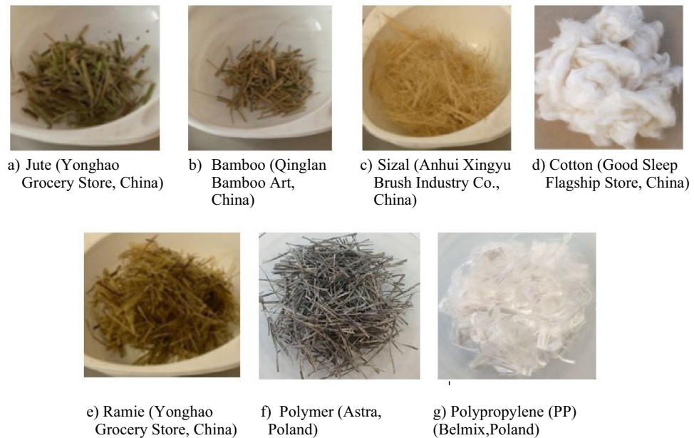
Figure 2. Fibre used in research [Fot. Y.Gu].
