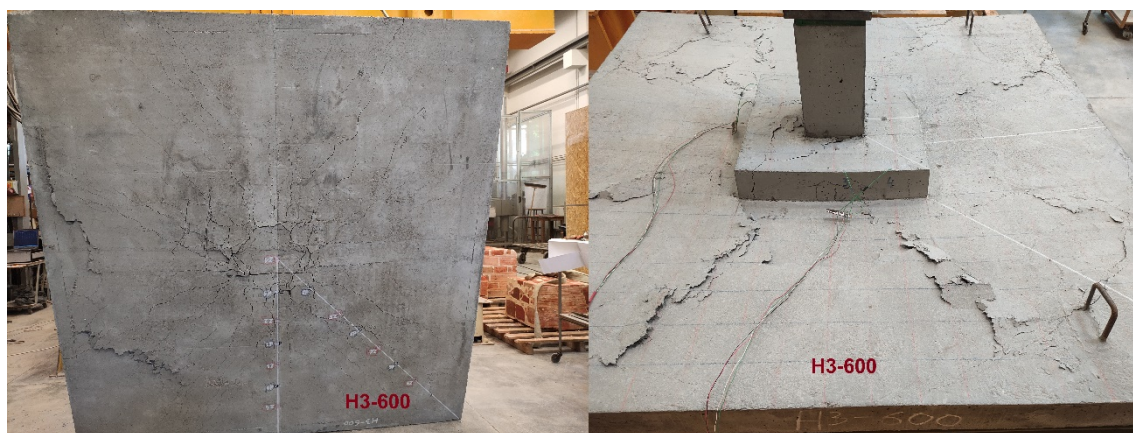
Fig. 9. Failure form of H3-600 element.
